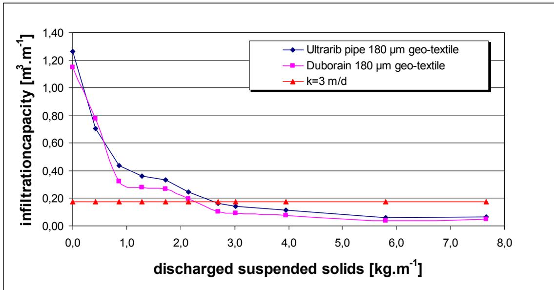
Figure 1. Relation pollution load - infiltration capacity
